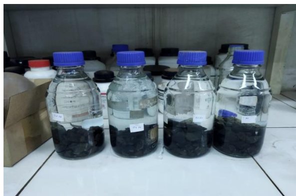
Figure 2. Nickel Slag Leaching Process Using Sulfuric Acid
