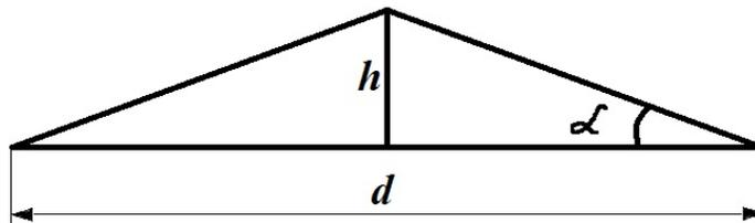
Figure1. By definition, the dynamic angle of repose
