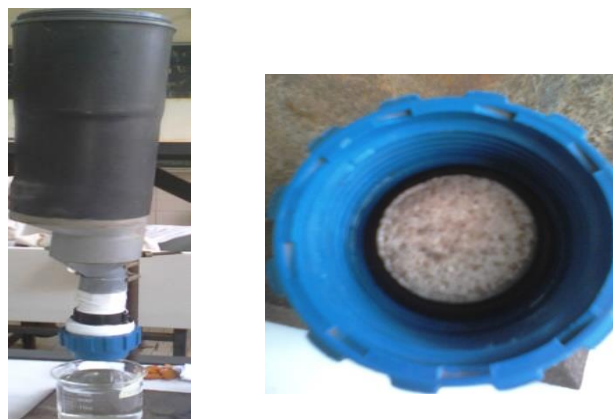
Figure 2: filter model optimum (having component proportions: 0.5 plastic, 0.25 sand, 0.25 porogen) fabricated by the two different methods: the melt moulding and the improved melt moulding porogen leaching technique
