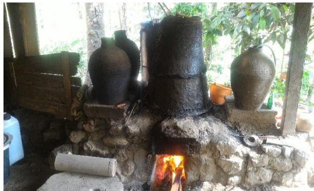
Figure 1. A traditional process of making arak
