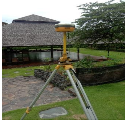
Figure 3. Setting up a GPS device for ground control point measurements
