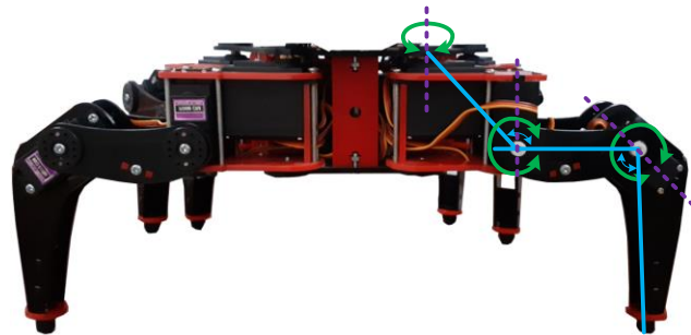
Figure 12. The angular motion of the servo motor on the hexapod robot leg
