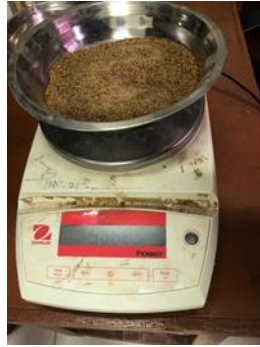
Figure 5. The process of checking the moisture content in fine-age
