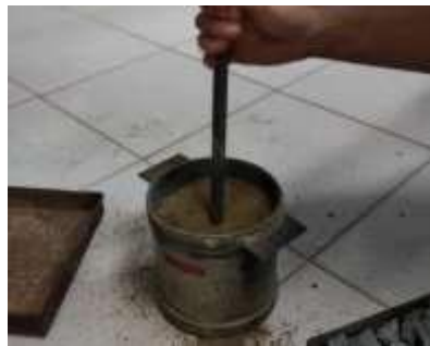
Figure 7. Fill weight testing process
