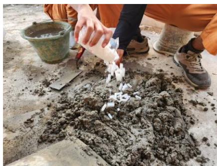
Figure 9. Process of mixing ABS material into mix/paving mixture Block
