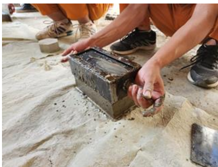
Figure 10. Paving block test specimen mould process
