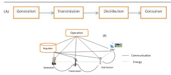
Figura 1. Conventional electrical infrastructure (A) and intelligent infrastructure (B)
