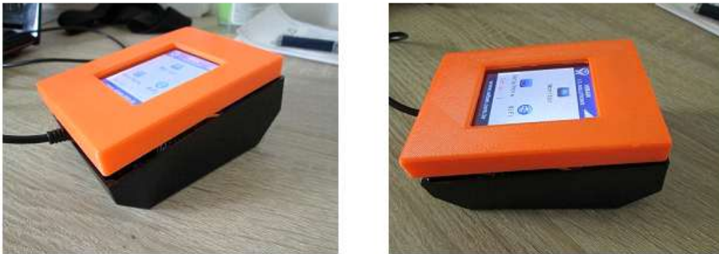
Figure 8 TF 3D object printed and coupled with the Nextion TFT, connected in the Patola PB-204/3 box
