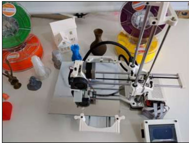
Figure 1. Stella 3D printer, selected for the printing of objects.
