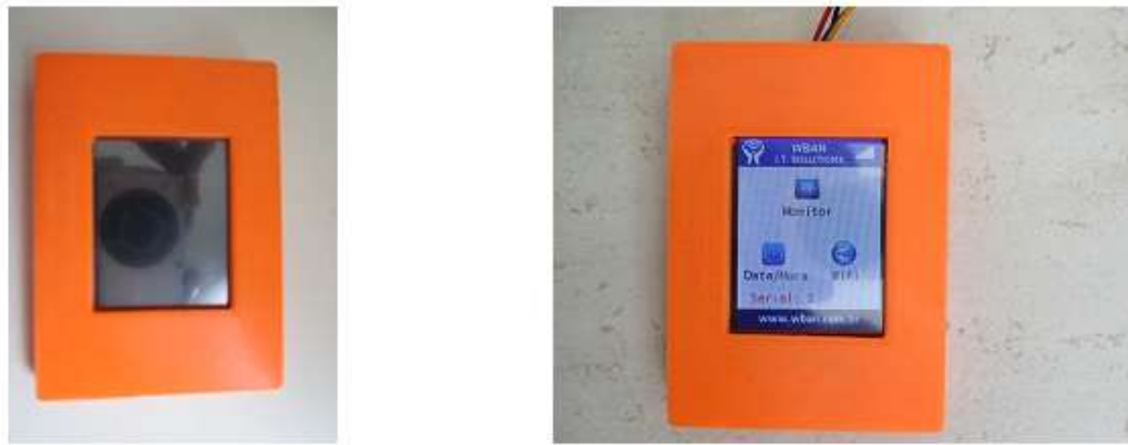
Figure 7 TF Nextion TFT device fixed to 3D object
